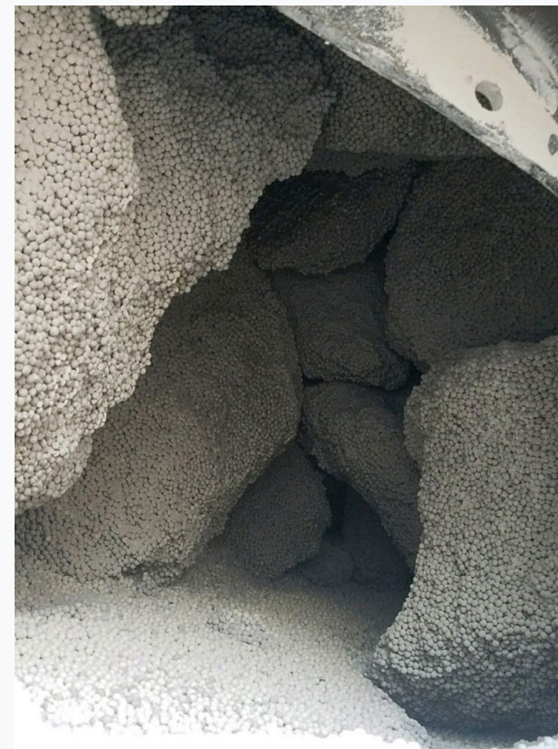
Agglomerated, channeled bed — flow short-circuits (diagram right)
