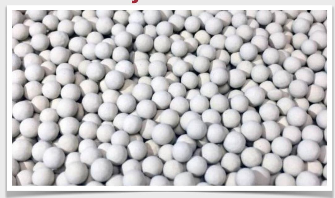
**L** thaDry® is a high-performance molecular sieve engineered for dynamic VPSA & TSA ethanol dehydration.
