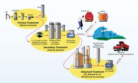
Landfill gas is a natural byproduct of the decomposition of organic material in landfills. This gas is composed of roughly 50% methane, 50% carbon dioxide, and a small amount of non-methane organic compounds. Landfill sites use various equipment and technology to treat this gas into achieving acceptable compositions of impurities for pipeline requirements. The treatment process of Landfill gas has three major stages:
