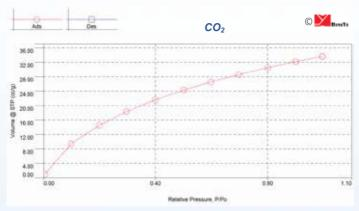
*HYGB500B* shows high CO<sub>2</sub> separation under a very low pressure, which lowers the consumption of oxygen during generation and improves economic performance.
