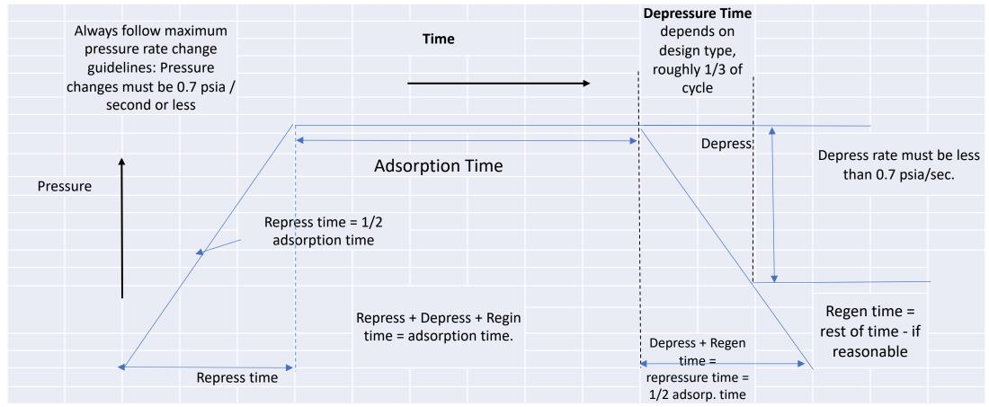
Adsorption time = mass feed rate of water/working capacity Repressure time = ½ of adsorption time (must be less than 0.7 psia/second) Depressure + regeneration time = ½ of adsorption time Depressure time is the time required to get down to around 20-25 psia Regeneration time is all the remaining time
